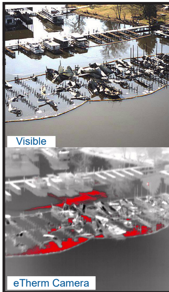
Visible and eTherm (Thermal + Polarization) images identifying oil spill after a marina fire near Huntsville, AL.
