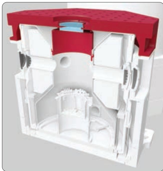
Cross-sectioned view of the OptiCool cryostat showing the Large Top-Volume Housing Kit installed. This provides an additional 57 mm of overhead beyond the standard sample volume.
